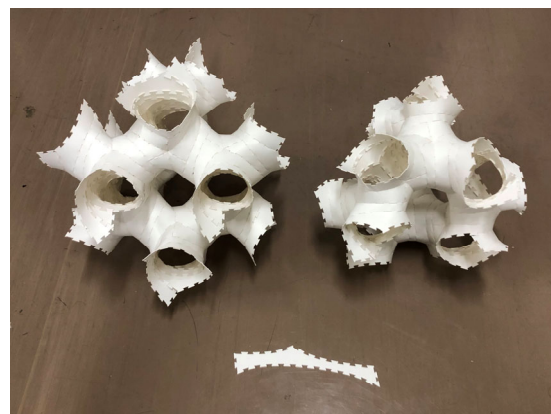
Figure 3 Physical prototype. Both D and G surfaces are assembled from single type of strip module.
